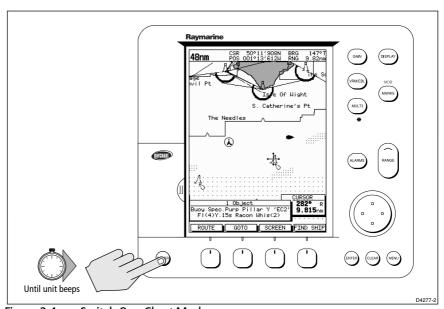
Figure 2-1: Switch On - Chart Mode
